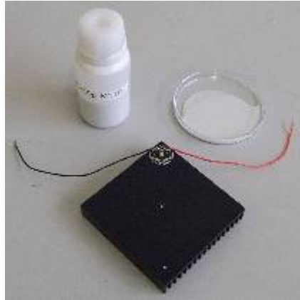
“COM-G52” and heat sink fin with a power LED bonded
